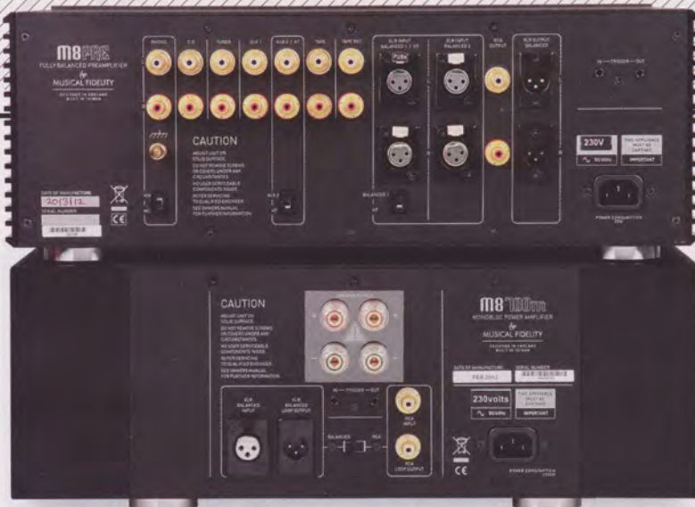
ABOVE: The pre and power are ideally connected via balanced XLRs – the M8700m even has a daisy-chained XLR output. In addition to two XLR ins, the M8PRE offers MM/MC phono, four line ins (inc. HT loop-through) and a tape in/rec out
